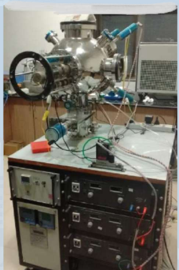
Metal Sputtering Unit
