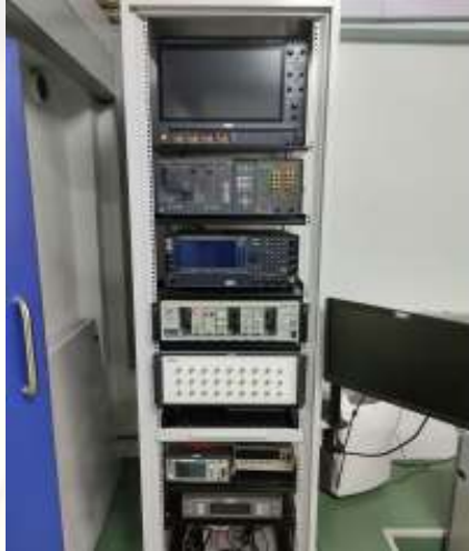
2. Oscilloscope, Arbitrary wave generator, Vector signal generator, Lock in amplifier , Keithley SMU
