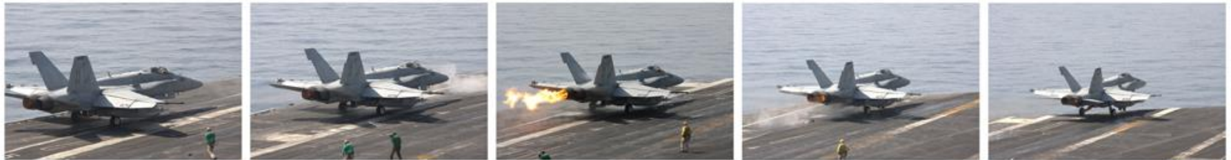
F-18C compressor stall during catapult launch - USS Nimitz - 19.10.09
