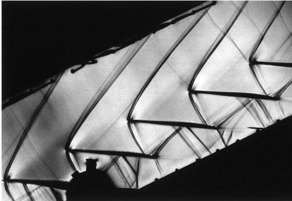
Transonic compressor cascade at M= 1.25
