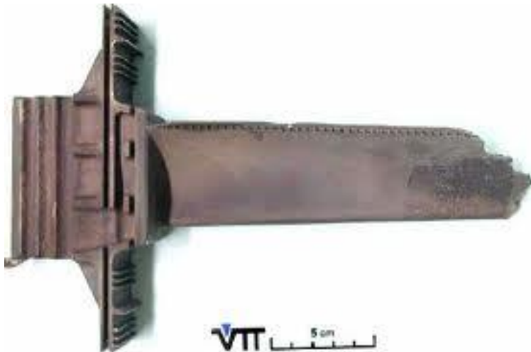
Trailing edge crack in the first stage turbine nozzle trailing edge.
