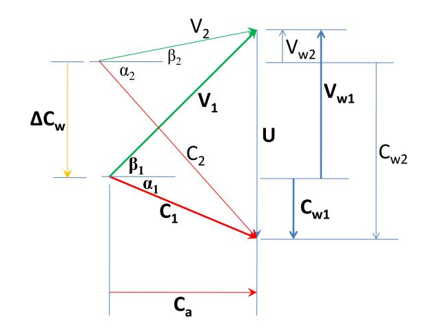
• Assuming  $C_a = C_{a1} = C_{a2}$ , from the velocity triangles, we can see that
