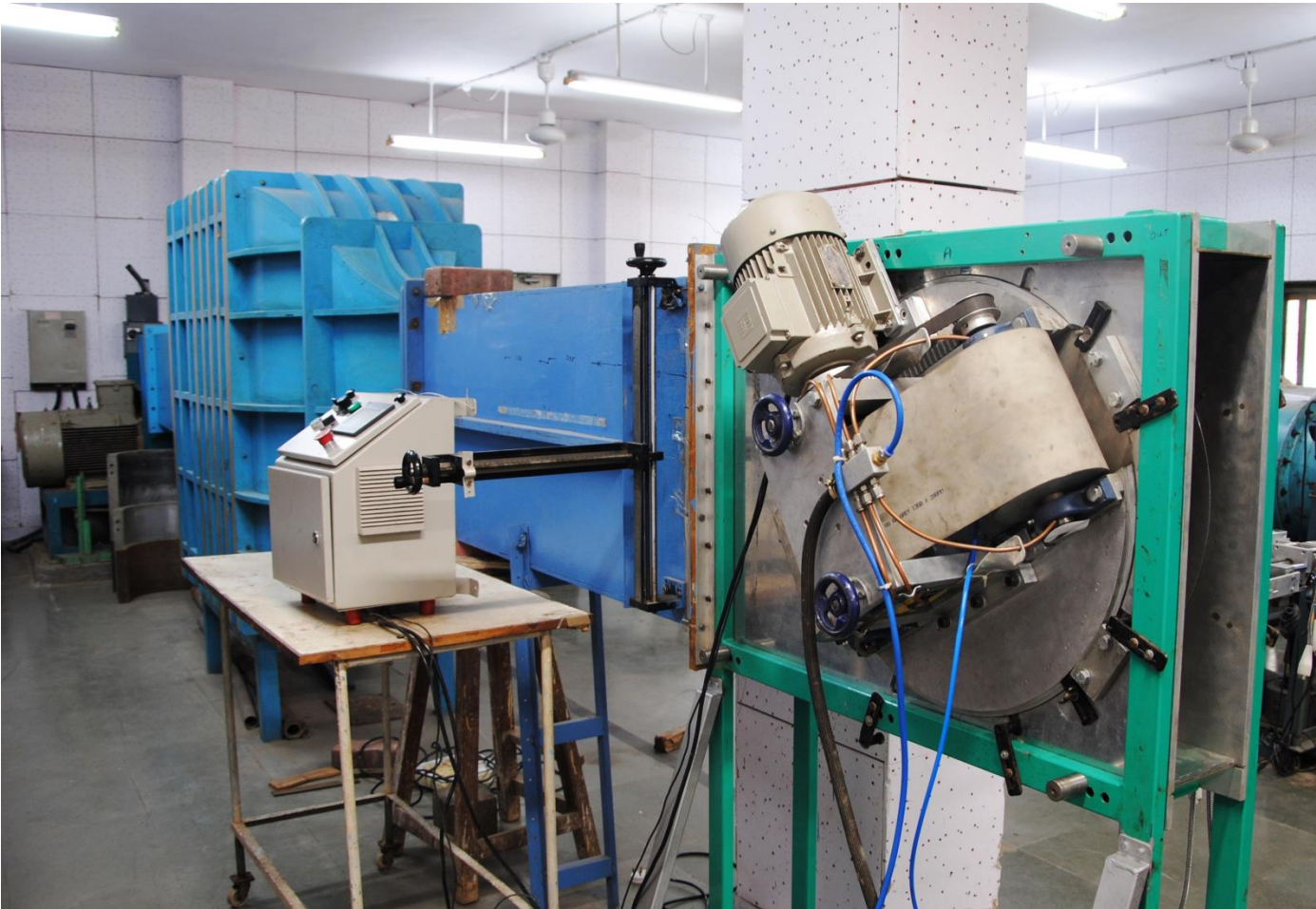
Low-speed Cascade Tunnel at the Turbomachinery Research Lab, IITB
